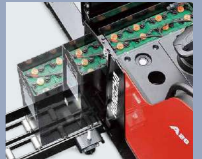
Side battery change is standard feature
